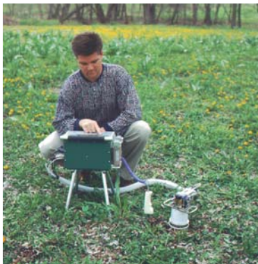
The LI-6400/6400XT console displays flux rate calculations in numeric and graphical form for evaluation in the field.
