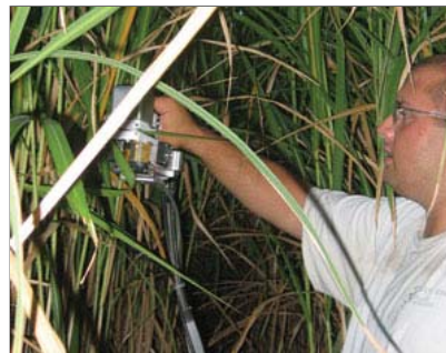
University of Illinois at Urbana-Champaign doctoral student Frank Dohleman uses the LI-6400 to make photosynthesis measurements in Miscanthus canopy.
