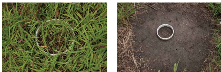
Figure 2. Natural (left) and bare (right) soil rings used to determine soil CO 2 fluxes at the IBDP site.
