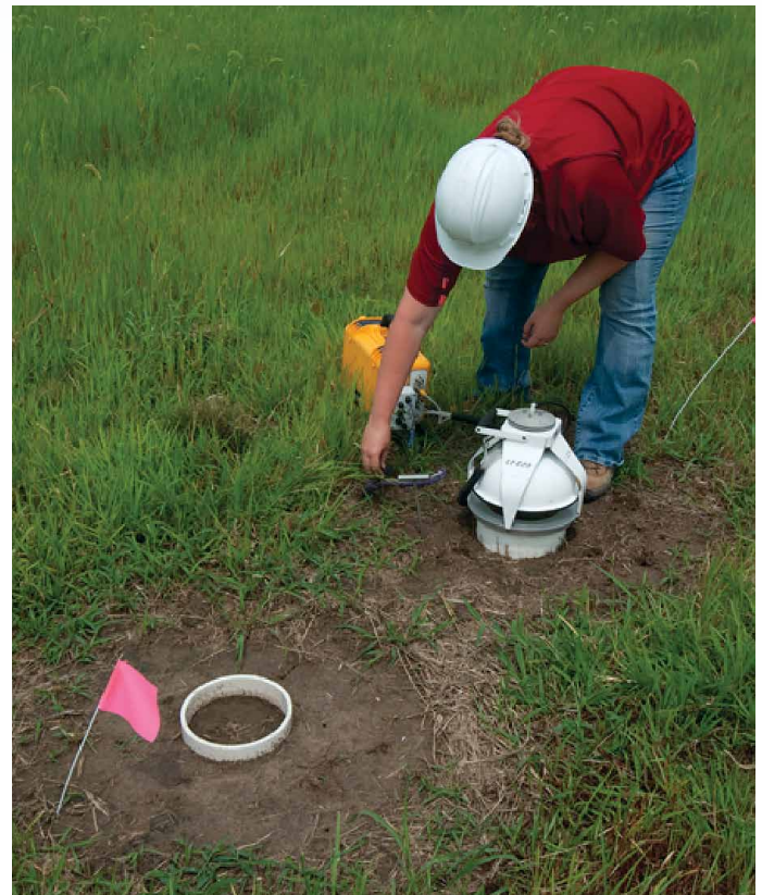
Figure 1. Measuring soil CO 2 fluxes at the IBDP site using the LI-COR LI-8100.
