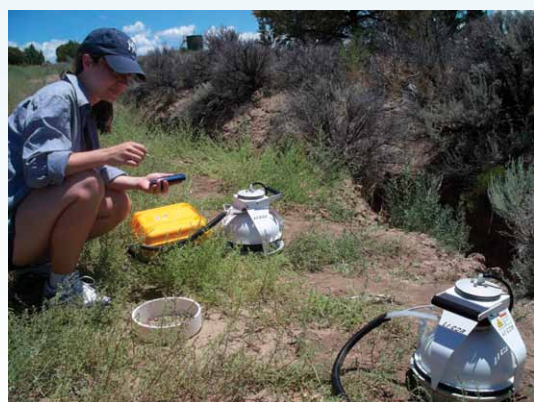
A RECS participant makes soil CO 2 flux measurements with the LI-8100 in New Mexico.
