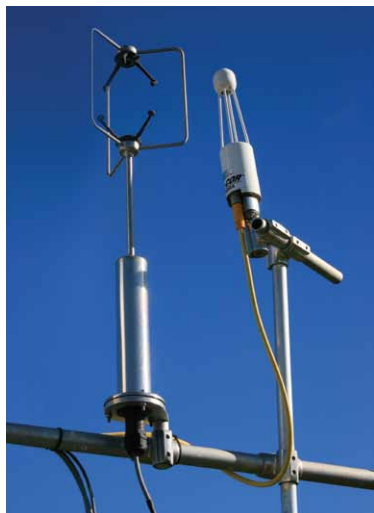
Figure 5. An example of the instrumentation setup for an Eddy Covariance flux measurement. Picture shows a 3-D sonic anemometer (Gill Windmaster™, Gill Instruments Ltd., Lymington, England) and an Open Path CO 2 /H 2 O analyzer (LI-7500A, LI-COR Biosciences, Lincoln, NE).
