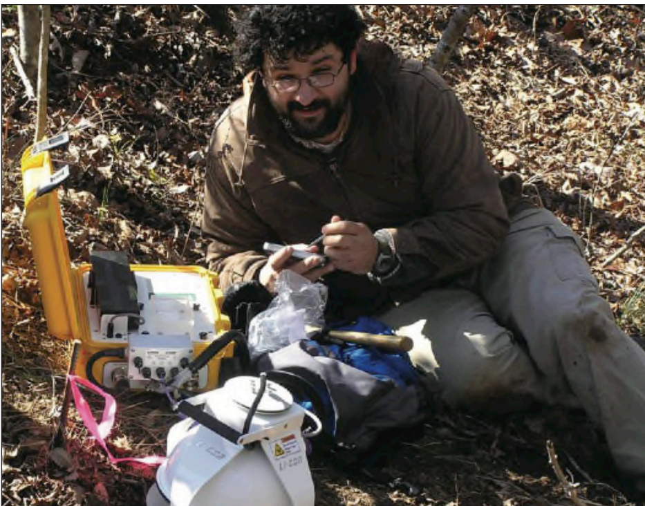
Adam Dayan, a graduate student at the University of Alabama, performs surface CO 2 monitoring with the LI-8100 and 8100-103 at the Black Warrior Basin test site.
