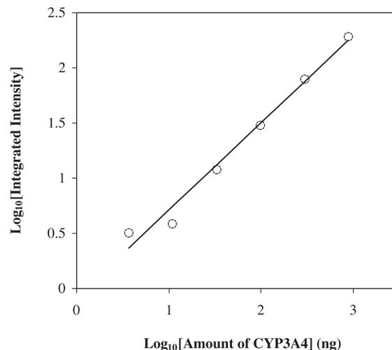
**Figure 3. Linearity of fluorescence detection.** The intensity of each CYP3A4 band (corresponding to 55 kDa molecular weight) was integrated with the LI-COR Odyssey software. The logarithm of CYP3A4 quantity is linear ( $R^2 = 0.98$ ) with respect to the logarithm of the fluorescence intensity signal.
