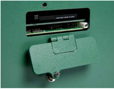
The expansion slot accepts either a Compact Flash card or the 6400-26 Ethernet adapter.
