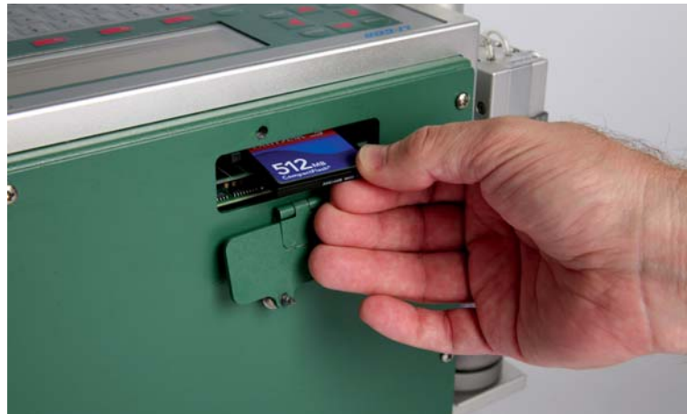
The expansion slot accepts either a Compact Flash card or the 6400-26 Ethernet adapter.
