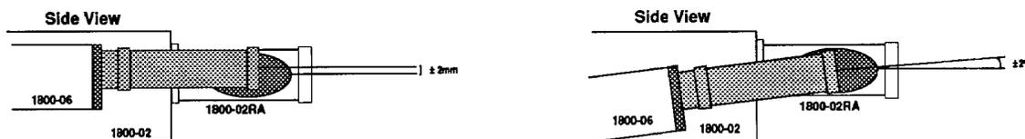
2. Orient the telescope lens tube at an angle of  $45^\circ (\pm 2^\circ)$  from the 1800-02RA accessory tube, when viewed from directly above the equipment. In the absence of a protractor or a square, a  $45^\circ$  angle can be made by folding a piece of paper across opposite corners.
