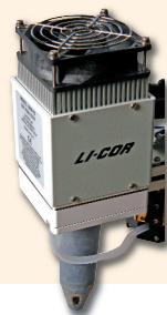
Figure 2. The RGB Light Source and WPA Chamber interface with the LI-6400XT Portable Photosynthesis System. Plant and container are sealed inside the WPA with an o-ring or flange to facilitate rapid assessment of individual plants. The top of the WPA seals to the chamber bottom with an airtight o-ring.
