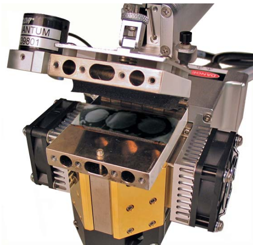
Figure 3. Place the strip of Propafilm over the 3 holes on the black spacer on the lower leaf chamber manifold...
