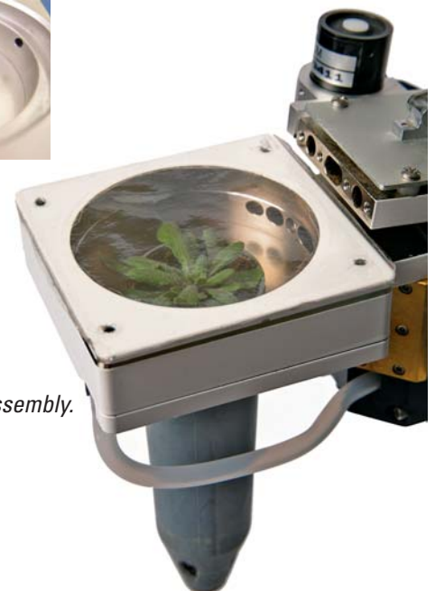
Figure 7. Install the standard exhaust tube, or exhaust tube with needle valve assembly onto the metal tubes shown.
