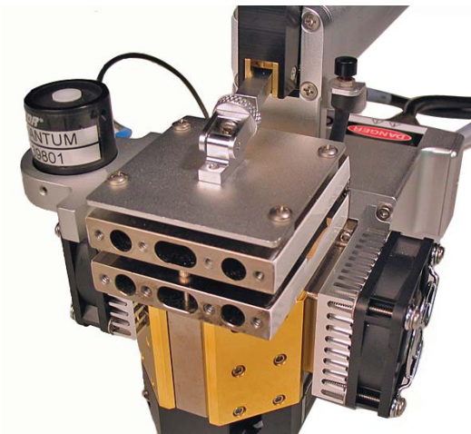
Figure 3. Place the strip of Propafilm over the 3 holes on the black spacer on the lower leaf chamber manifold...
