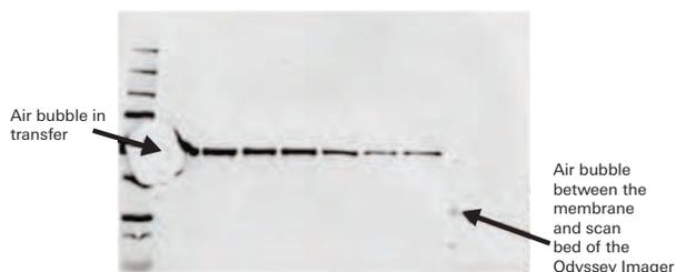
**Figure 6. Air bubbles affect image appearance.** Examples of bubbles in the transfer sandwich or on the Odyssey Imager scan bed.
