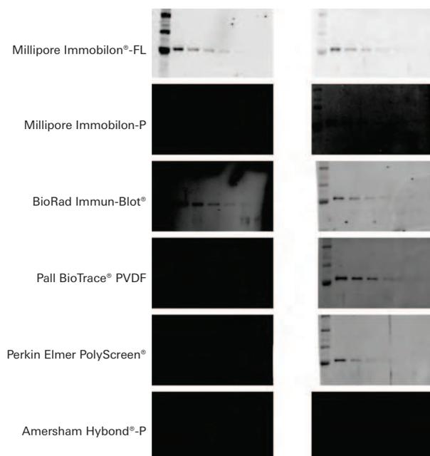
**Figure 1. Membrane autofluorescence from PVDF affects Western blot performance.** Transferrin was detected by Western blotting, using various vendors and brands of PVDF membrane. Blots were imaged with the Odyssey Classic Infrared Imaging System in both 700 and 800 nm channels.
