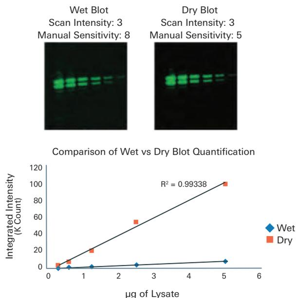
**Figure 7. Scanning of wet and dry Western blots.** The same Western blot was scanned wet and dry with an Odyssey Classic Imager. Optimal image display settings are shown. Quantification (graph below images) demonstrates higher signal intensity on the dry blot.
