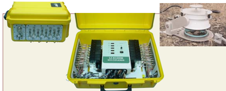
Figure 1. 16-chamber multiplexing system control box. The top two panels show one side of the control box with 8 gas ports and a soil CO 2 flux chamber.
