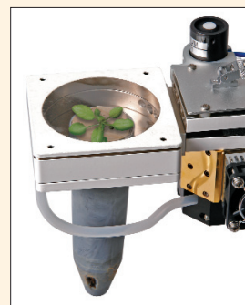
Figure 1. Whole Plant Arabidopsis Chamber mounts to LI-6400/LI-6400XT Portable Photosynthesis System. Plant and container are sealed inside with an airtight O-ring or flange to facilitate rapid assessment of individual plants.
