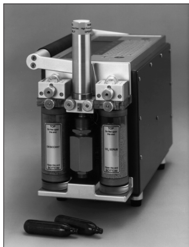
Figure 2. CO 2 source assembly mounted on LI-6400.
