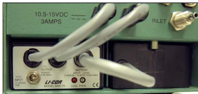
Figure 1. The 6400-70 AC Module fits in a battery compartment in the console. If you install a battery in the other compartment, and plug it into the module (as shown at left), that battery will trickle charge, but more importantly, provide continued operation for 1-2 hours in the event of a mains power failure.
