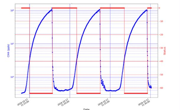
The LI-7810 was tested against higher concentrations of CH<sub>4</sub>. The instrument responded and continued to measure, however, specifications are not guaranteed outside of the 0 – 50 ppm range for CH<sub>4</sub>. This is reflected in the status codes given at higher concentration measurements.
