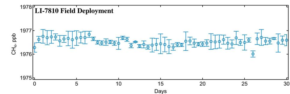
Located in an enclosed shelter, the analyzer measured ambient air between stability checks. During stability checks, the analyzer was flushed for 10 minutes with tank gas\*\* and a time series data set was subsequently recorded for 10 minutes every 12 hours. The figure shows the mean value of the 10-minute measurements. Error bars represent a 1 $\sigma$  confidence interval (68%).
