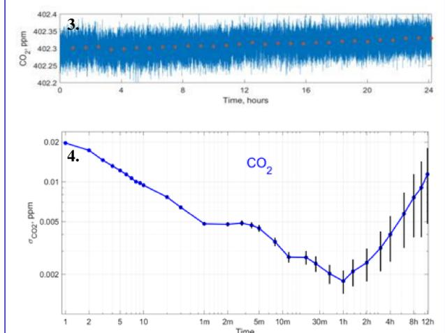
Chart 3: The instrument was operated continuously over a 24-hour period with a continuous flow of tank gas. The blue line shows 1-second measurements; the orange line shows a 50 minute block average.
