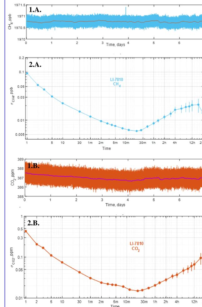
Chart 1: The instrument was operated continuously over a 7-day period with a continuous flow of tank gas. The blue line shows 1-second measurements; the orange line shows a 50 minute block average. Chart 1.A. reflects the high precision CH<sub>4</sub> data set, with chart 1.B. providing the CO<sub>2</sub> data from the same instrument. The LI-7810 provides high precision CH<sub>4</sub> measurements, with CO<sub>2</sub> data similar to other IRGAs available.
