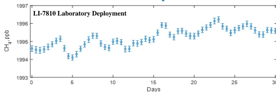
The analyzer measured ambient air between stability checks. During stability checks, the analyzer was flushed for 10 minutes with tank gas\*\* and a time series data set was subsequently recorded for 10 minutes every 12 hours. The figure shows the mean value of the 10-minute measurements. Error bars represent a 1 $\sigma$  confidence interval (68%).
