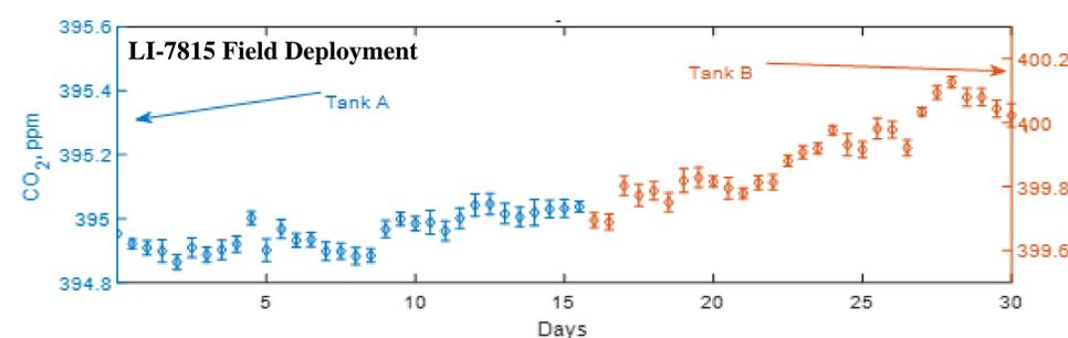
Located in an enclosed shelter, the analyzer measured ambient air between stability checks. During stability checks, the analyzer was flushed for 10 minutes with tank gas\*\* and a time series data set was subsequently recorded for 10 minutes every 12 hours. The figure shows the mean value of the 10-minute measurements. Error bars represent a 1 $\sigma$  confidence interval (68%).
