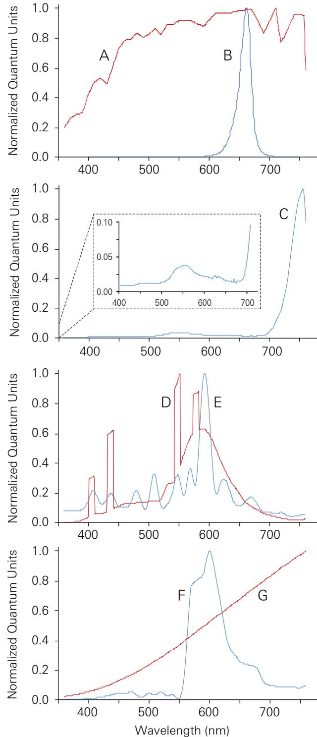
**Figure 3.** Spectra of light sources used in calculating sensor errors, photon units ( $\mu\text{mol m}^{-2} \text{s}^{-1} \text{nm}^{-1}$ ) normalized to the maximum: (A) open sky<sup>1</sup>; (B) red LED, 660 nm peak; (C) daylight under soybean canopy; (D) cool white fluorescent; (E) metal halide; (F) tungsten halogen<sup>2</sup>; and (G) high pressure sodium.
