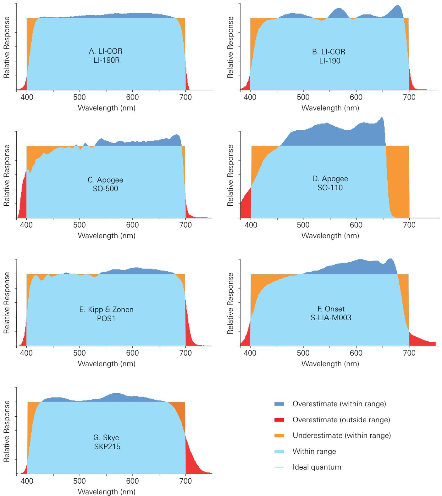
**Figure 4.** Comparison of the spectral responses of seven sensors to the ideal response. Sensitivity of each sensor is normalized so that the total overestimate equals the total underestimate between 400 and 700 nm. Spectral response curves are for one representative sensor.
