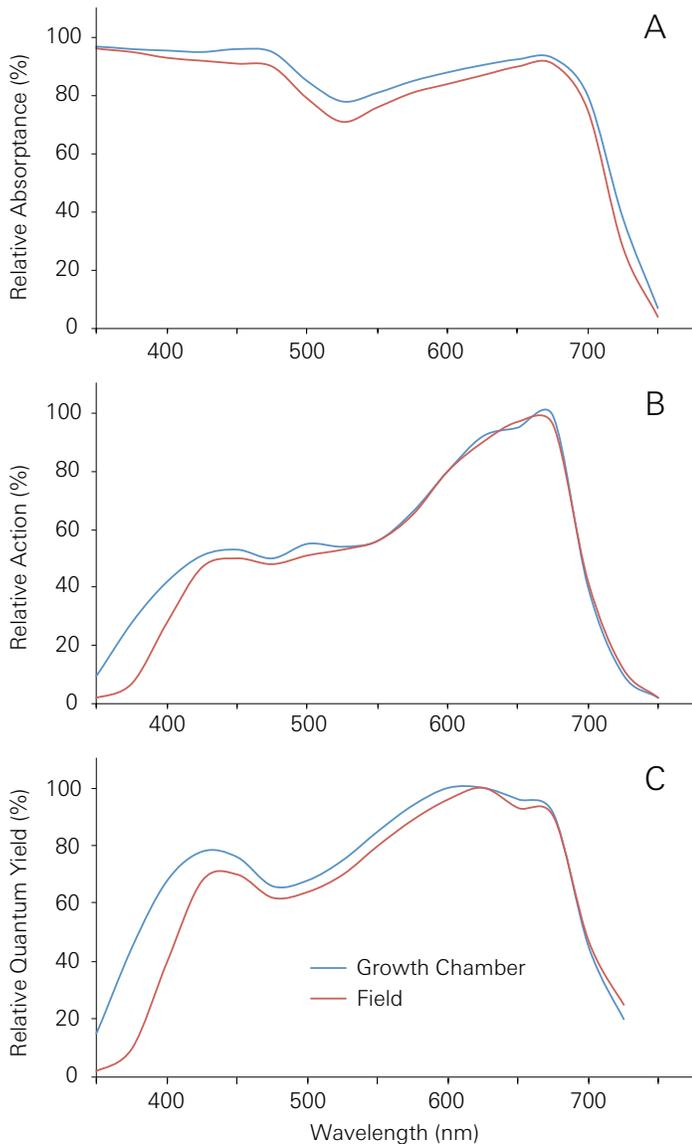
**Figure 1.** For leaves grown in the field and in a growth chamber, normalized (A) leaf absorbance spectra, (B) leaf photosynthetic action relative to incident light energy, and (C) leaf photosynthetic yield relative to number of photons absorbed (from McCree 1972a).
