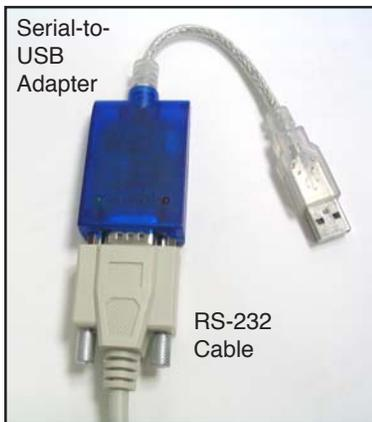
2. Plug the USB end of the adapter into a USB port on the host computer, and the RS-232 cable into the LAI-2000. Power the LAI-2000 on. The first time that you connect the LAI-2000 to the computer using this adapter you will see a "Found New Hardware" message:
