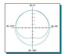
Figure 2. Typical Angular Response of the LI-193SB Spherical Quantum Sensor.
