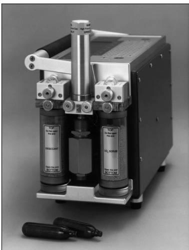
Figure 2. CO 2 source assembly mounted on LI-6400.
