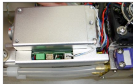
Figure 7. Reattach the log button cable connector as shown.
