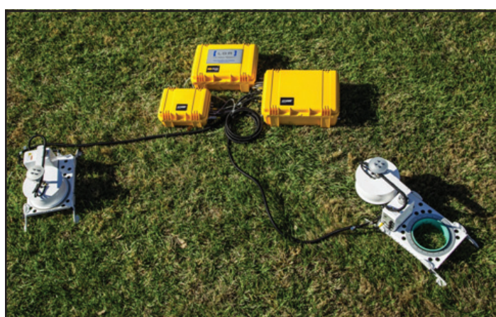
Figure 1. A multiplexed LI-8100A System deployed with the Los Gatos Research Ultra-Portable Greenhouse Gas Analyzer (model 915-0011).
